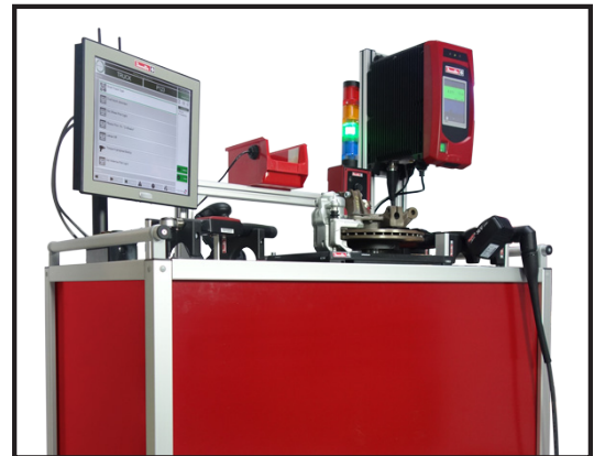
A set up including torque transducers and torque joint kits alongside a torque data collector is common for regularly auditing production assembly tools on the factory floor.
