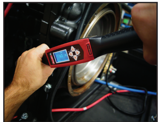
A digital torque wrench with a built-in data collection system being used to test the torque readings of a typical joint on a car engine.
