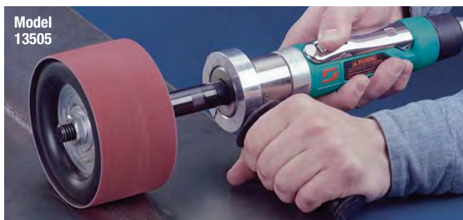
13505 Dynastraight® powers optional 94472 Dynacushion® pneumatic wheel.
