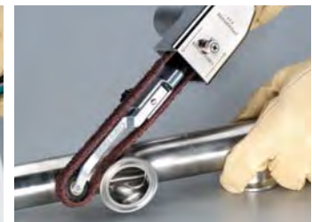
Clean and finish using non-woven nylon belts.
