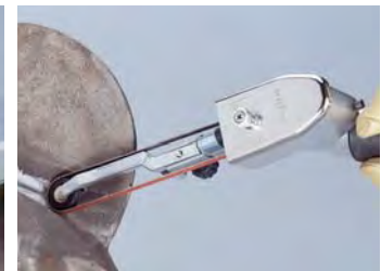
Optional 11204 Contact Arm offers ability to grind into contours.
