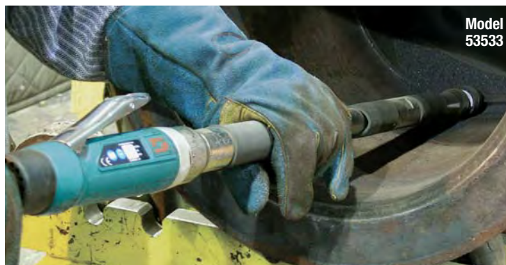
Extend into hard-to-reach places by choosing the suitable extension for the job.
