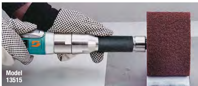
13515 Dynastraight® sets grain pattern in stainless steel.
