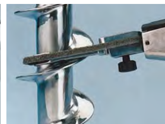
Clean and finish using non-woven nylon belts.
