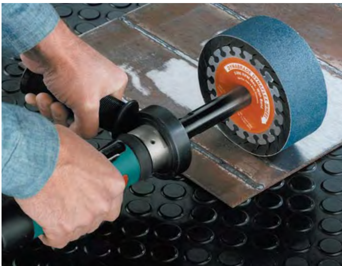
Dynabrade Dynastraight® and Die Grinder models powering Abrasive Bands.
