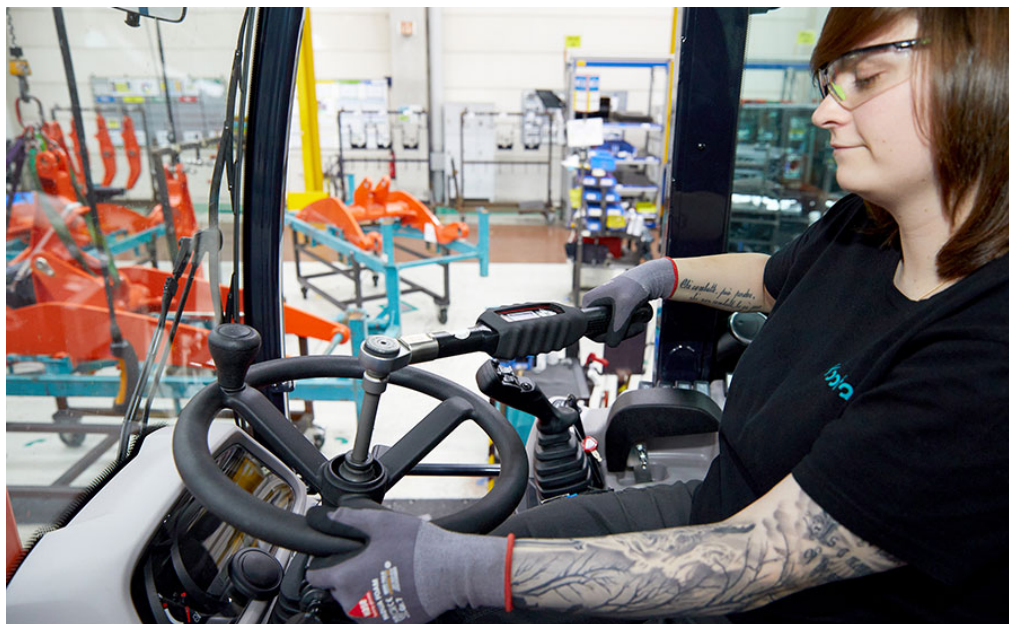
An assembler installs the steering wheel on a wheel loader. Photo courtesy Desoutter Industrial Tools
