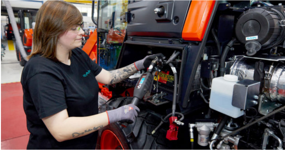
The ground screw on the engine main switch is tightened with a digital torque wrench. Here, the screw must be tightened to 8.8 to 11.8 newton-meters. Photo courtesy Desoutter Industrial Tools
