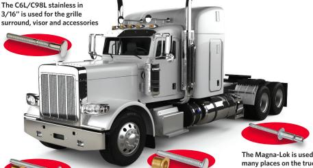
The 3/16" Magna-Grip is used for the hood and fender, body panels and sleeper
