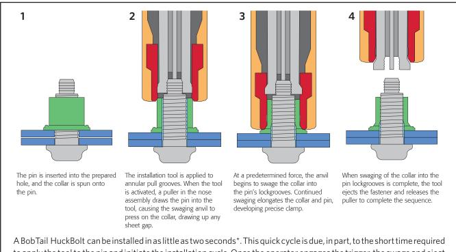
A Bob I all HuckBolt can be installed in as little as two seconds\*. This quick cycle is due, in part, to the short time required to apply the tool to the pin and initiate the installation cycle. Once the operator engages the trigger, the swage and eject sequence is programmed to complete the cycle without any additional installer input.
