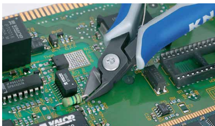
Cut with 79 42 125 (without bevel)
