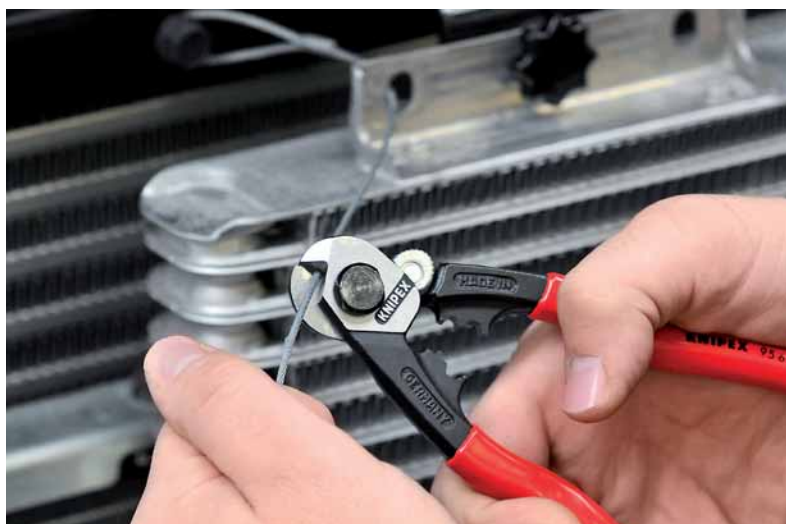
Crimping of the end ferrule onto the traction cable
