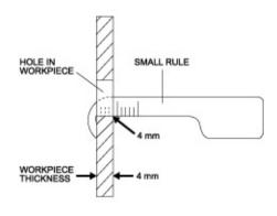
**NOTE:** The SMALL RULE is specially designed to measure the WORKPIECE Thickness.
