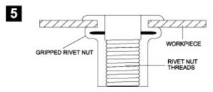
The RIVET NUT is therefore gripped in the WORKPIECE firmly and the RIVET NUT Threads are built up securely.
