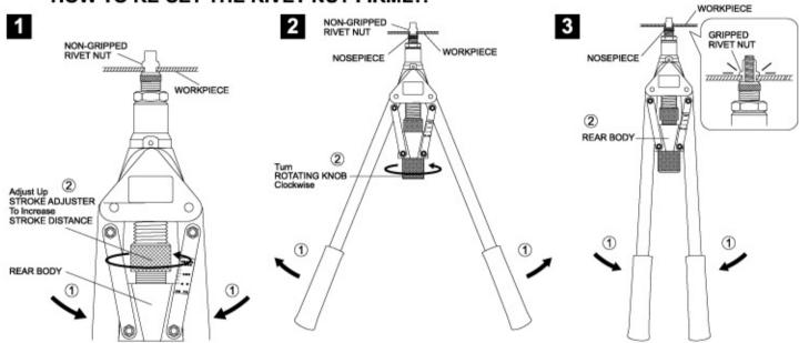
Still hold to squeeze 2 HANDLES to touch REAR BODY ①, adjust the STROKE ADJUSTER upward to increase the Stroke Distance 1.0mm or 0.04" step by step to try ②.
