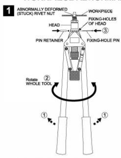
Open 2 HANDLES a little bit ①, rotate whole TOOL to align the FIXING-HOLES of HEAD with the inside LONG FIXING-HOLE of MANDREL SEAT ②, then plug the FIXING-HOLE PIN Into these FIXING-HOLES and put the PIN RETAINER onto FIXING-HOLE PIN End ③, the free rotation of THREADED MANDREL is therefore stopped.
