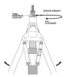
Finally use SERVICE WRENCH to fasten NOSEPIECE LOCK NUT by turning Clockwise.
