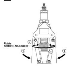
Close 2 HANDLES completely ①, rotate STROKE ADJUSTER ② to adjust the proper Stroke Distance in 2 popular ways.
