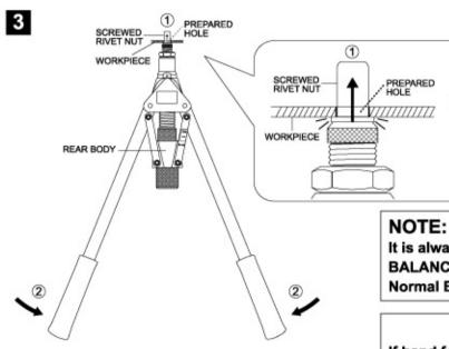
Insert the Screwed RIVET NUT into the Prepared Hole of WORKPIECE to touch WORKPIECE ①. Squeeze 2 HANDLES to touch REAR BODY ②, that drives THREADED MANDREL downwards to deform RIVET NUT a Bulge against the back of WORKPIECE to fasten RIVET NUT in the WORKPIECE ③.
