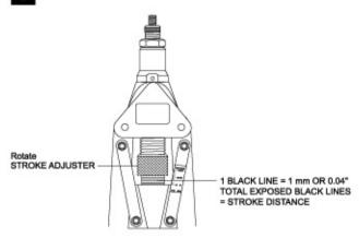
Second Way: Rotate STROKE ADJUSTER to find out the Total Exposed Black Lines of the STROKE INDUCATING LINES:
