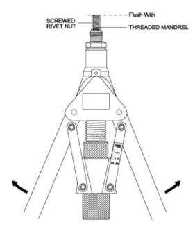
**NOTE:** After adjusting the Protruding Length(L) of THREADED MANDREL, the Screwed RIVET NUT should be flush with the THREADED MANDREL.
