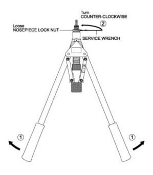
Open 2 HANDLES fully ①, use SERVICE WRENCH to loose NOSEPIECE LOCK NUT by turning Counter-Clockwise②.
