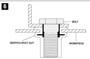
Complete the fastening work with a Bolt screwed to the Gripped RIVET NUT.
