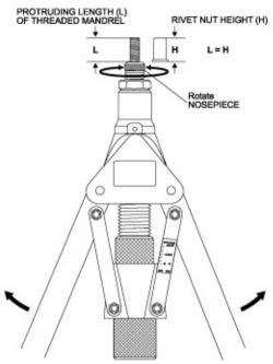
Use Hand to rotate NOSEPIECE to adjust the Protruding Length (L) of THREADED MANDREL to be same as the RIVET NUT Height (H), L = H.
