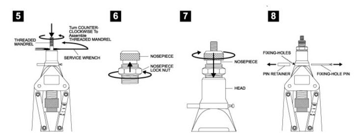
Use Hand and SERVICE WRENCH to assemble the working size of THREADED MANDREL into MANDREL SEAT firmly by turning Counter-Clockwise.
