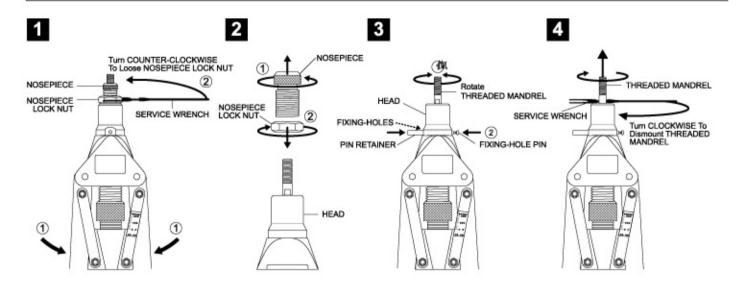
Close 2 HANDLES completely ①, use SERVICE WRENCH to loose NOSEPIECE LOCK NUT by turning Counter-Clockwise ②.
