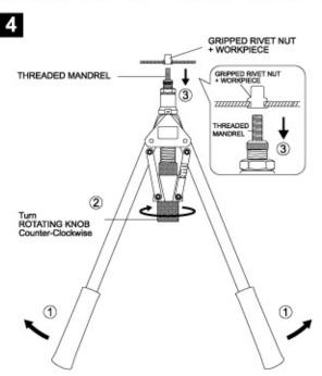
Open 2 HANDLES fully ①, turn ROTATING KNOB Counter-Clockwise ② to unscrew THREADED MANDREL from the Gripped RIVET NUT completely ③.
