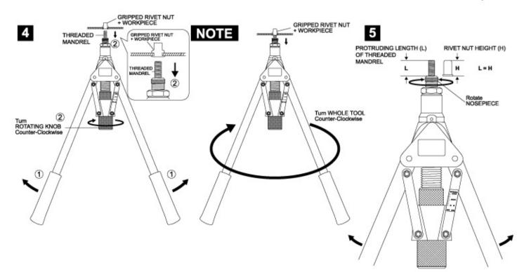
Open 2 HANDLES fully ①, turn ROTATING KNOB Counter-Clockwise to unscrew THREADED MANDREL from the Gripped RIVET NUT and WORKPIECE ②. NOTE: If the THREADED MANDREL still can not unscrew from the Gripped RIVET NUT and WORKPIECE, turn whole TOOL Counter-Clockwise to unscrew THREADED MANDREL completely.
