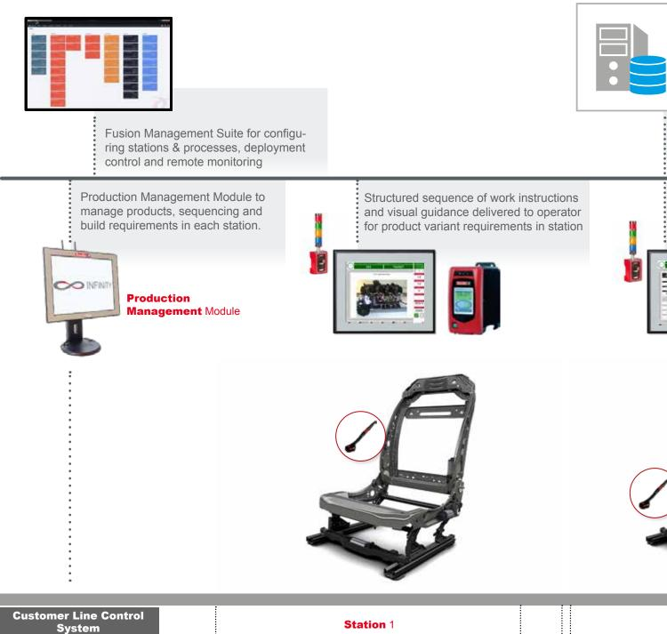
Integration with line control systems for data exchange, product in station, line run-
