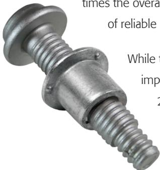
While the "holding power" of HuckBolts is a key characteristic, these lockbolts also offer several important time-saving features. To begin, installation of these fasteners usually requires less than 2 seconds, and special indicator notches on the base of a HuckBolt collar provide a quick visual confirmation of an accurate installation. Additionally, using these advanced fasteners saves time since they never need retightening or re-torqueing, even in the most vibration-intensive application.
