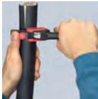
Turning the tool for circumferential cut
