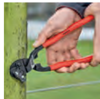
Two-hand operation for maximum cutting force
