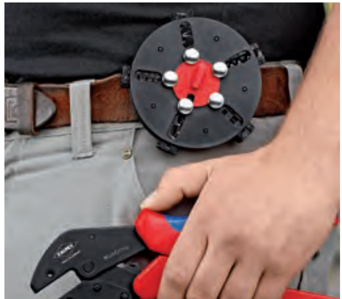
Magazine for crimping dies can be carried on a belt
