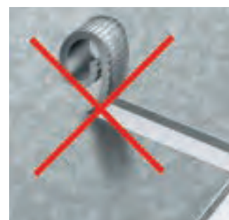
Notching without chip breaking
