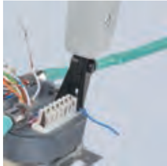
Inserts and cuts cables in one operation
