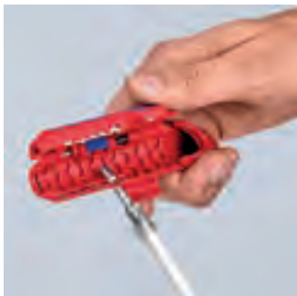
Stripping of a coax cable
