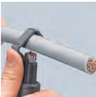
Setting the tool for circular cut
