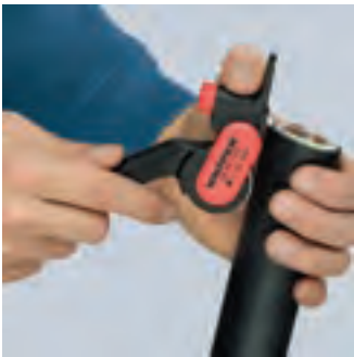
Setting the tool for longitudinal cut
