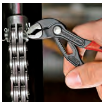
Teeth set against the direction of rotation have a self-locking effect and prevent slipping on the workpiece.
