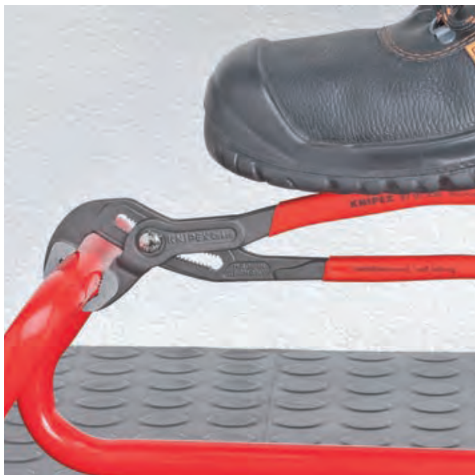
Teeth set against the direction of rotation have a self-locking effect and prevent slipping on the workpiece.
