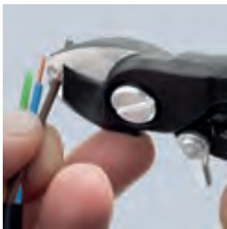
95 41 165: with stripping function
