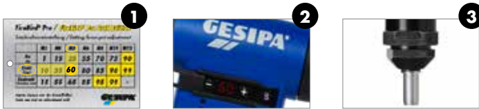
Setting force guide – Example: Steel M5
