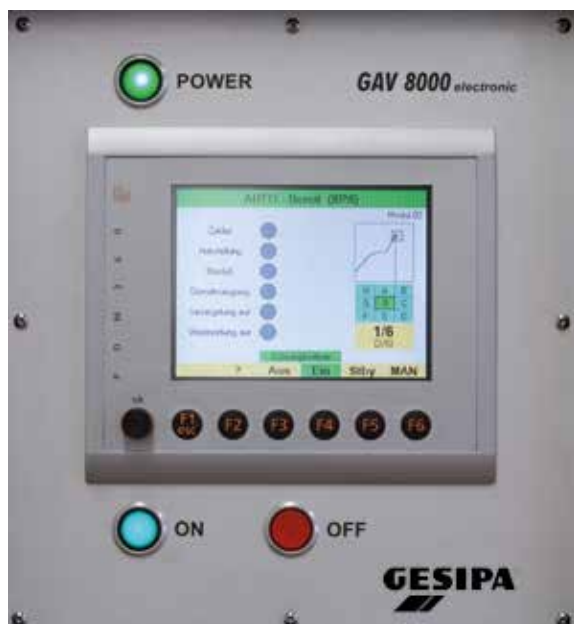
Display of a GAV 8000 electronic indicating the setting curve as part of the setting process monitoring
