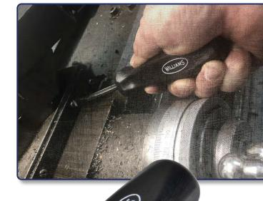
**Hex bolsters** on shafts allow a wrench to be used for extra turning power
