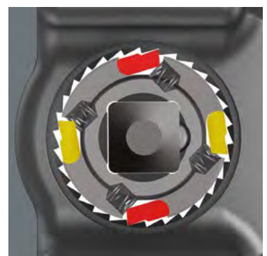
Dual ratchet teeth: gives the robust 30 saw teeth the precision engineering effect of 60 fine teeth with a 6° return angle.
