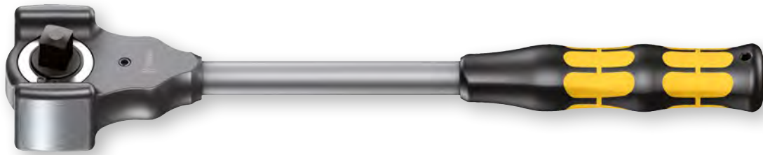
Changing the ratchet direction using a hardened push-through square drive ensures great resilience, since there is no susceptible switching mechanism that could be damaged by hammer blows. This is far more robust than a forward/reverse switch.
