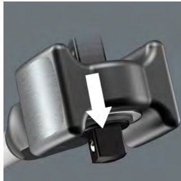
Changing the ratchet direction using a hardened push-through square drive ensures great resilience, since there is no susceptible switching mechanism that could be damaged by hammer blows. This is far more robust than a forward/reverse switch.
