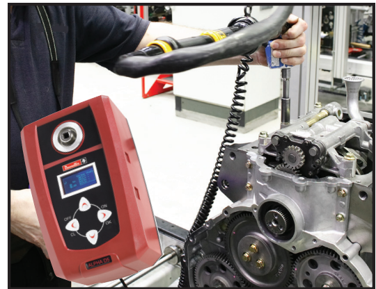
Torque tightening readings being audited with a torque data collector during the assembly stage of a large engine.
