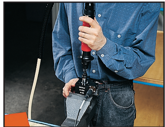
Power tool torque auditing takes place on and around the production line during the assembly process.
