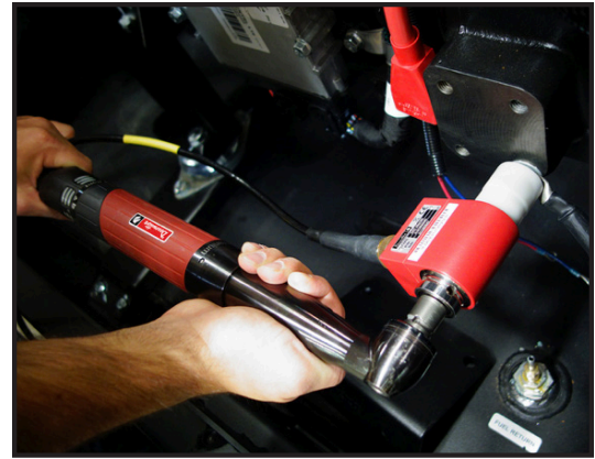
A rotary torque transducer and torque data collector being used during a quality audit test of a joint and fastener within the ag industry.
