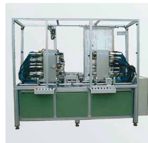
23 placing heads to assemble a computer chassis
