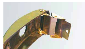
Composite material latch for wheel cover
