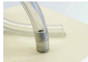
Grovit fastener used as a quick connect low pressure bleed hose
