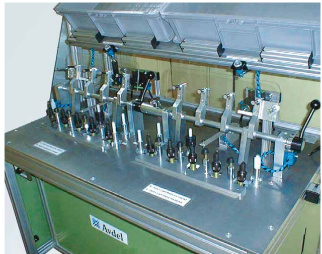
10 placing heads to assemble automotive sealing strips
