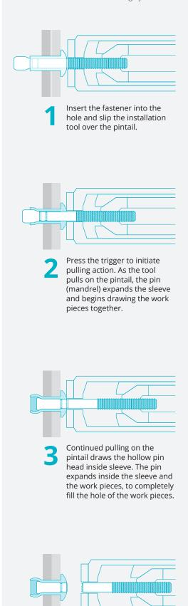
A solid circle lock between the pin and sleeve is formed just prior to the pin breaking flush with the sleeve head, completing the installation. 4 Huck<sup>®</sup> | Magna-Lok<sup>®</sup>
