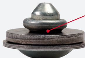
The Competition Bulb forms irregularly above sheet line resulting in lower installed values.
