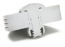
Lock groove on pin engages shoulder on rivet head, while the support ring "double locks" the pin within the bulb.
