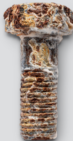
Hot dip galvanized bolt
