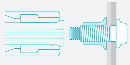
When swaging of the collar into the pin lockgrooves is complete, the tool ejects the fastener and releases the puller to complete the sequence.
