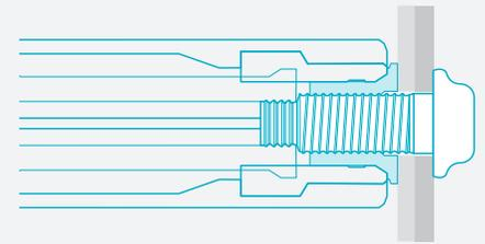
At a predetermined force, the anvil begins to swage the collar into the pin's lockgrooves. Continued swaging elongates the collar and pin, developing precise clamp.
