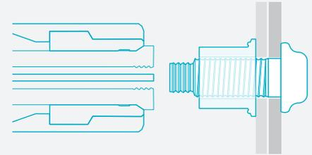
Insert pin into the prepared hole, spin the collar onto the pin.
