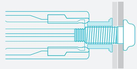
The installation tool is applied to annular pull grooves. When the tool is activated, a puller in the nose assembly draws the pin into the tool, causing the swaging anvil to press on the collar, drawing up any sheet gap.
