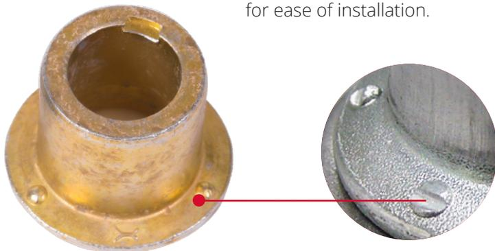
“Dots” on the BobTail collar indicates a full swage when at least one is crossed by the swage anvil.
