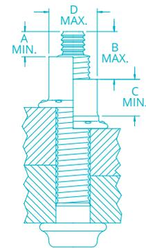
Should "A" or "B" dimensions exceed the given values, the fastener is out-of-grip. A "C" dimension less than the given value indicates an incomplete swage. A "D" dimension greater than the given values indicates an incorrect or worn anvil on the installation tool.
