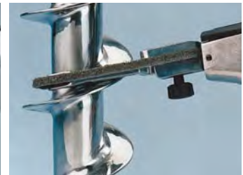
Clean and finish using non-woven nylon belts.
