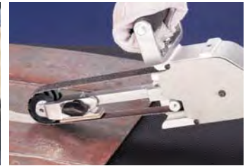
Model 11476 grinds weld seam and leaves in-line scratch pattern.
