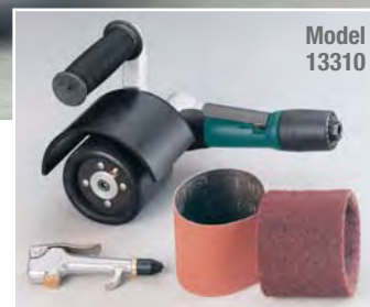
13300 Mini-Dynisher powers optional 94507 Dyncushion® pneumatic wheel on stainless steel.
