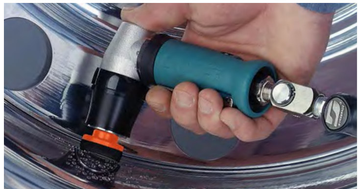
58035 Denibber shown with optional 95745 Speed Control.
