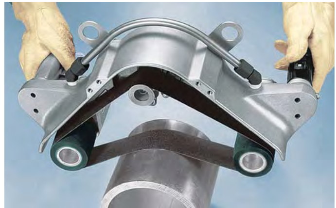
14300 Dynangle® II is utilized for "strap polishing" on a cylindrical stainless steel surface.
