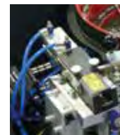
Escapement sensors Control/Secure escapement mechanism
