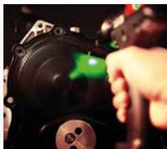
Shed light of OK/NOK directly on the application
