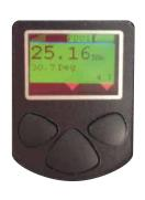
Tightening result on the OLED display
