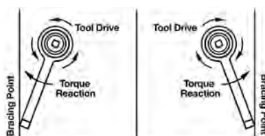
Torque Bar Opposes Rotation of Tool
