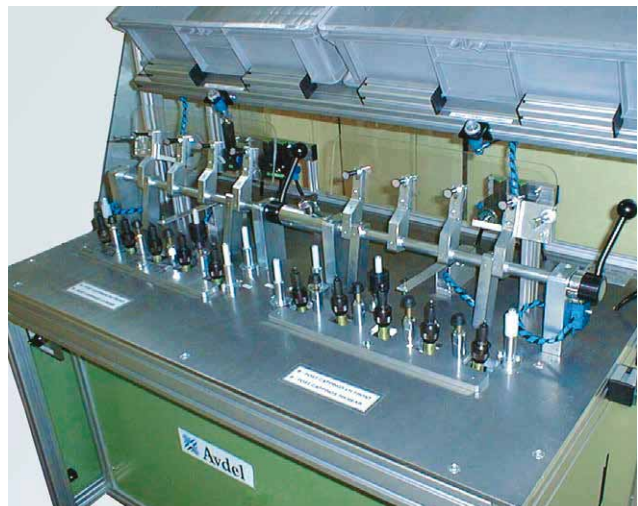
10 placing heads to assemble automotive sealing strips
