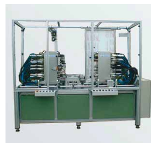
23 placing heads to assemble a computer chassis
