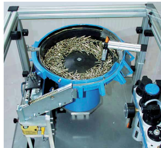
Fasteners are transferred from the bowl feeder to the placing head via the blow feeder
