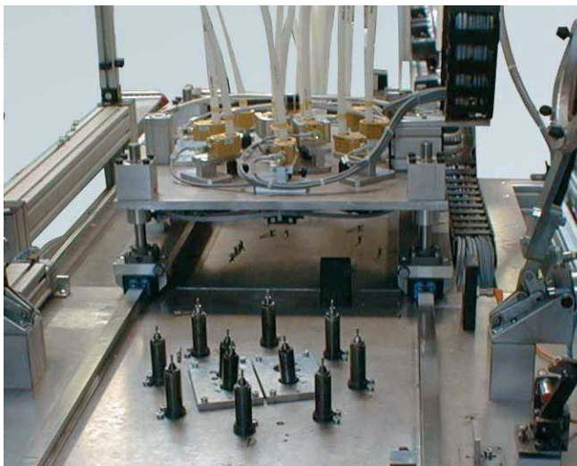
12 rivets placed in one assembly cycle
