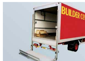
Column tail lifts
