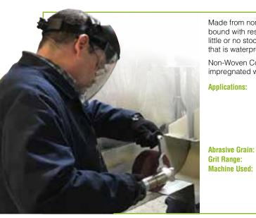
Made from non-woven synthetic fiber mesh, which is impregnated with abrasives and bound with resins, non-woven wheels are designed to create desired surface finish where little or no stock removal is required. Non-woven wheels have an open mesh construction that is waterproof, washable, conformable and non-loading.
