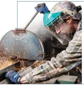
A chop saw is a light, low-horsepower portable machine. Although very similar to a compound miter saw, it is designed for cutting denser materials, like metal bar, tubing or pipe. Chop saw cut-off wheels are designed specifically for this machine with finer grit, softer grades, and reinforcement layers that match the application.
