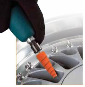
Spiral rolls are strips of abrasive cloth rolled and glued to form a solid shape that is designed to break down during use and reveal the next layer of abrasive.
