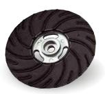
Air-Cooled Standard Back-up Pad Slotted hub design and curved ribs draw heat away from the grinding zone, reducing disc loading and increasing life. All pads have a 5/8"-11 threaded female hub for mounting. We also offer
