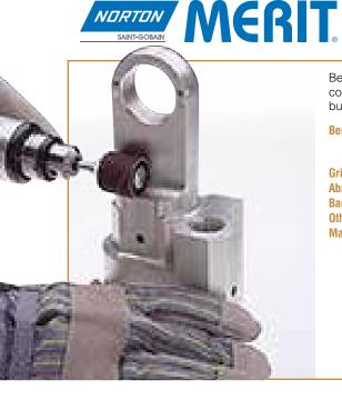
Best product for blending and polishing contours when smooth running is a primary concern. Used for finishing hard-to-reach areas, removing parting lines, imperfections, and burrs on all surfaces.
