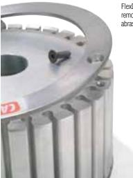
FlexDrum hub end plate removes for easy loading of abrasive segments.
