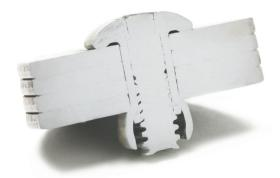
Lock groove on pin engages shoulder on rivet head, while the support ring "double locks" the pin within the bulb.
