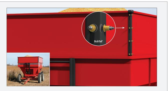
High strength, fast and easy installation, along with unmatched vibration-resistance, are what make HuckBolts<sup>\*</sup> the smart choice for heavy equipment assembly applications for agriculture.
