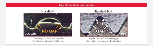
When compared with conventional nuts and bolts, HuckBolts have a much larger cross-sectional area and larger root radius, resulting in a much stronger and more secure joint. In fact, HuckBolts have up to 30% more bolt cross-sectional area, and up to 5x larger root radius than regular bolts, depending on the bolts used.
