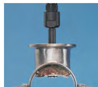
Sand and deburr inside small dia. pipe and other hard to reach areas with 3/4" – 1-1/2" stars.
