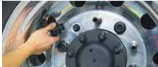
STEP 7 Install the nuts by hand.
