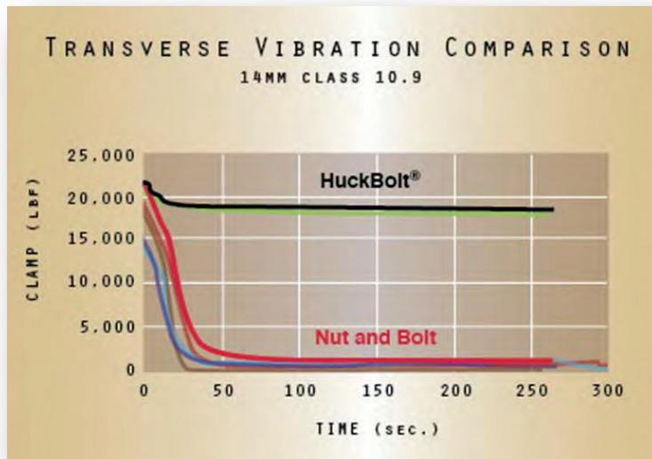
It should be noted that HuckBolts are not designed to replace all welds. These fasteners do leave a protrusion, which may not be acceptable for some applications. However, there are many applications where welding has been traditionally employed, in which HuckBolts are a viable alternative. Engineered for easy installation, and long, reliable life, these direct-tension HuckBolts can be a faster, more cost efficient, and safer alternative to traditional welding processes.
