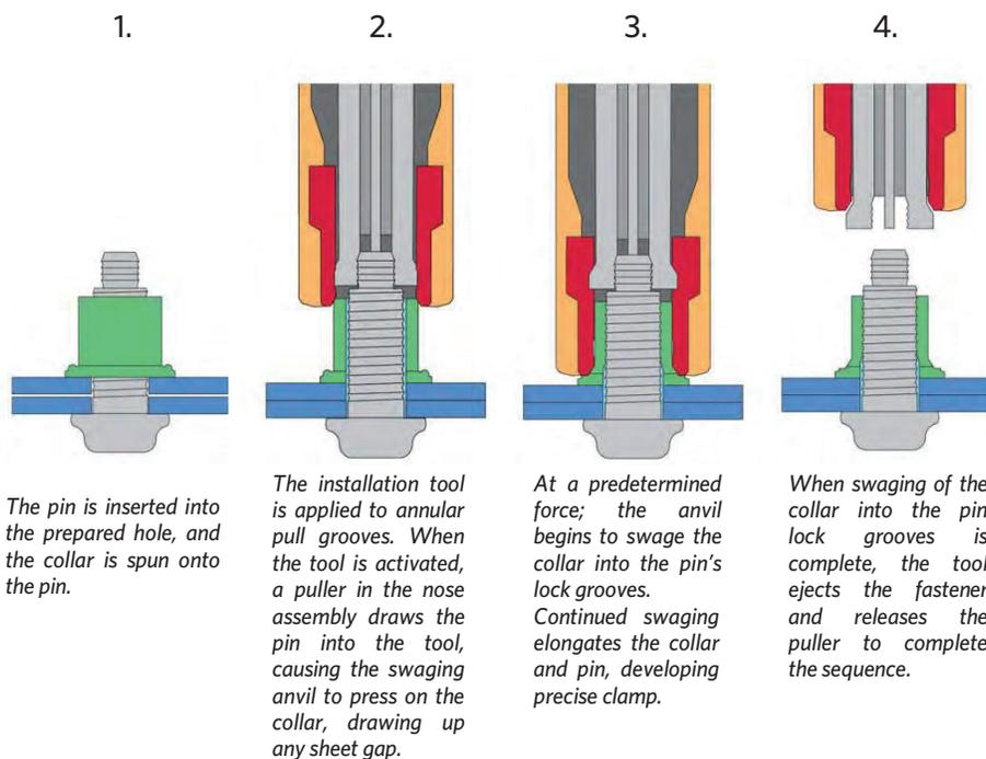
A BobTail® HuckBolt can be installed in as little as two seconds\*. This quick cycle is due, in part, to the short time required to apply the tool to the pin and initiate the installation cycle. Once the operator engages the trigger, the swage and eject sequence is programmed to complete the cycle without any additional installer input.
